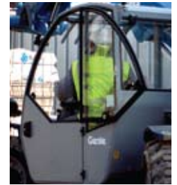
DOOR IN TWO SECTIONS: STEEL LOWER, GLASS UPPER. EACH SECTION CAN OPEN INDEPENDENTLY.
